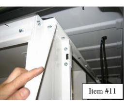
In the upper corner of each side of the 3<sup>rd</sup> Compartment Doorframe are small filler panels that need to be installed. Attach using ½" x ¾" carriage bolts, washers, and serrated
